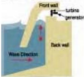
Oscillating Water Column
