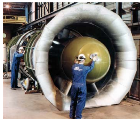
Figure 15. Turbo generation system - Trial Assembly
