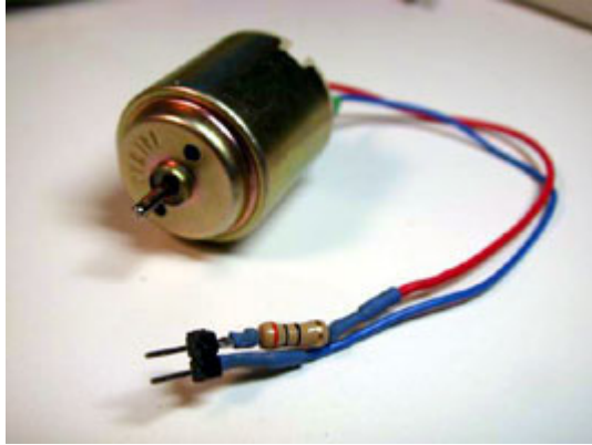
Example of a motor with a power limiting resistor
