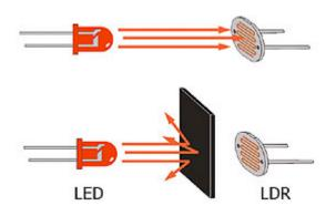
There is another idea to accomplish the same task. You can beam light outwards and measure the amount of light that is reflected back. When there is nothing to block the light, the reflected light will be very small. However, if an object blocks the light, it reflects more the light back. This is what we call a **reflective light sensor**. The benefit of this kind of sensor is that the sensor is located all in one place and no alignment is needed when you change the direction of the sensor.
