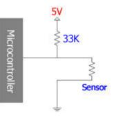
Now, we know that if the voltage drop is 5v, we get a reading of 1023. We can use the same equation to determine the sensor readings directly.
