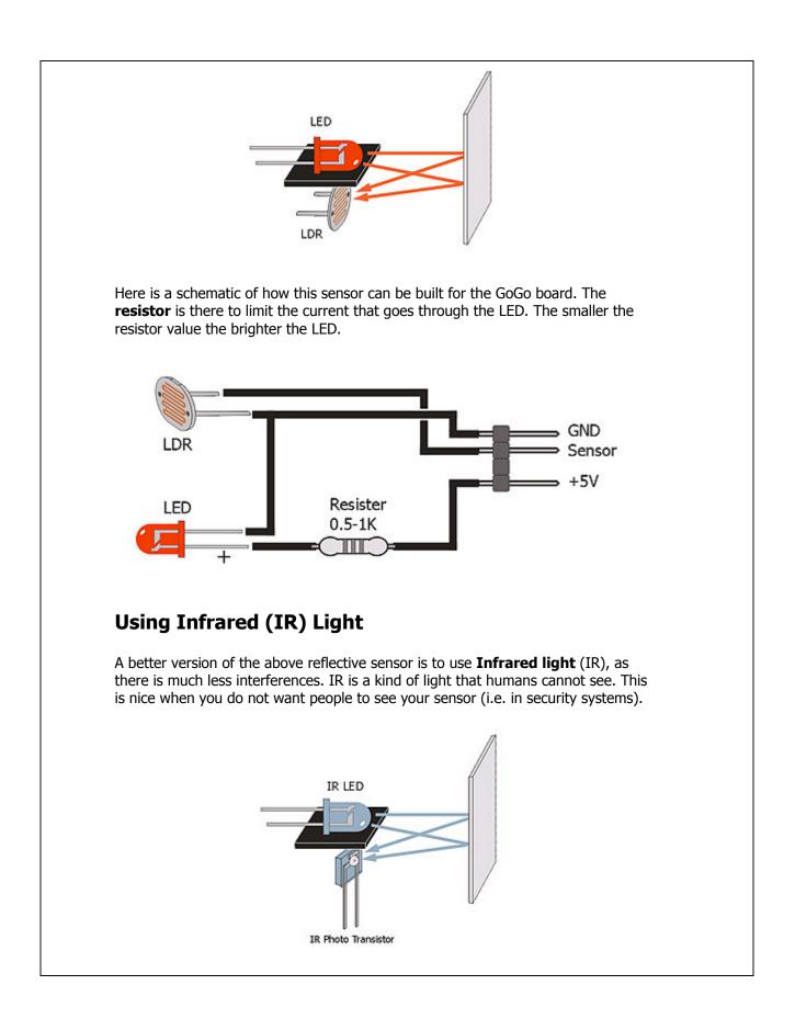
Notice in the diagram that we use an **IR phototransistor** instead of the LDR. In this case, the two functions the same way, but the IR phototransistor is much more sensitive to IR light than an LDR. The following is a schematic of how to build this sensor.
